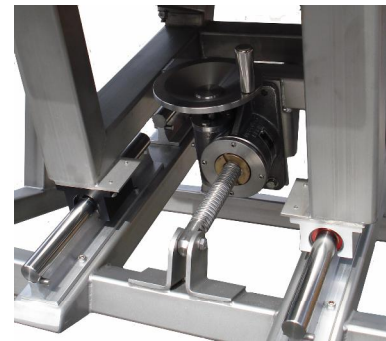
Mechanical x-ray view adjustment for optimum detection performance.
