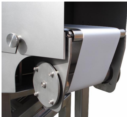
Small diameter end roller enables smooth conveyor-to-conveyor transfer.
